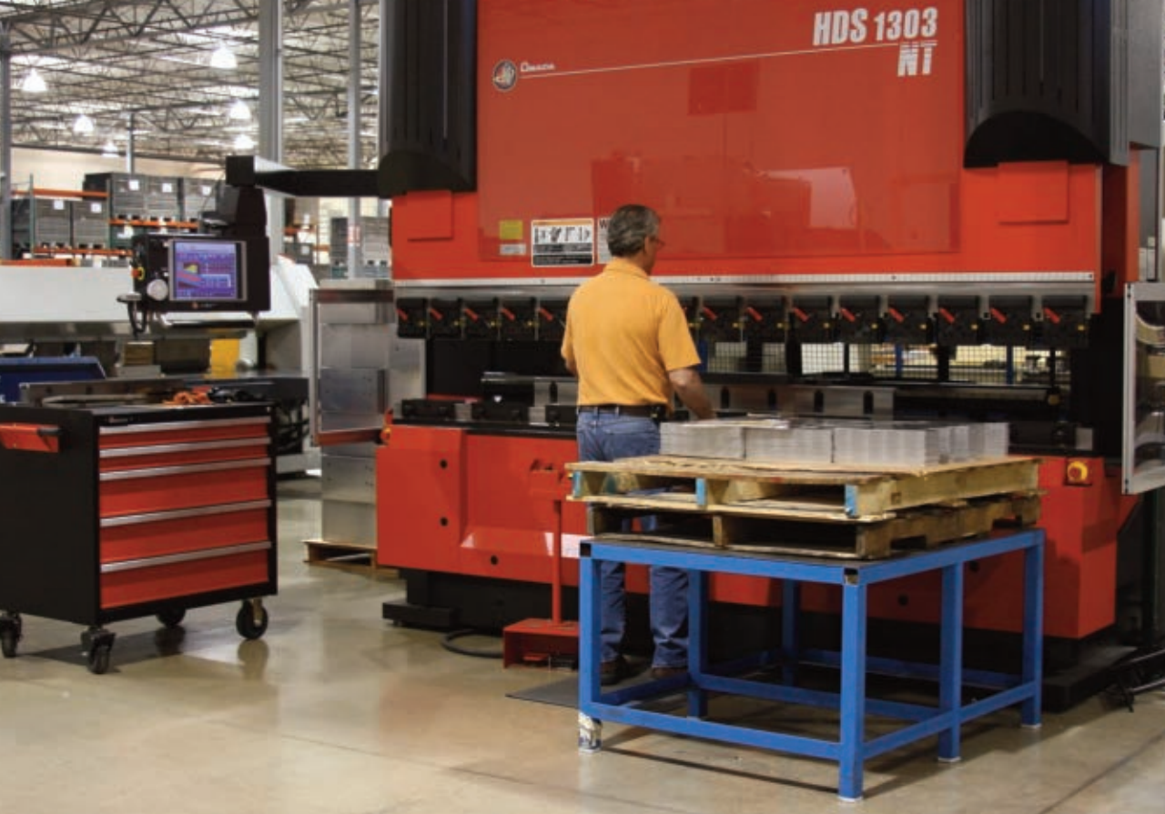
Figure 1 An operator at Quality Fabricators can retrieve a program that was sent to the control from offline bending software. Photo courtesy of Quality Fabricators.
